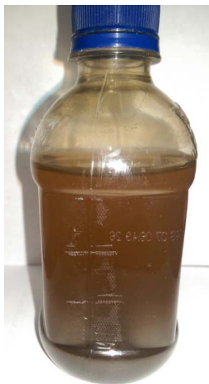
Figure 4. Water containing elevated levels of manganese sampled from a residence.
